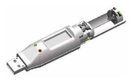
While the tab is pushed down, gently pull apart the two parts of the data logger enclosure.
